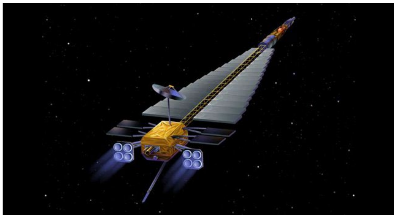
Figure 4: Project Prometheus was a 200 kWe nuclear reactor powered space craft, designed to reduce travel time from Earth to Mars to weeks. The project was abandoned in 2006, after significant development. [11]
